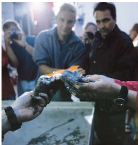
7.11 > A group of marine scientists on the deck of a research vessel ignite methane gas released from a degrading hydrate block.
